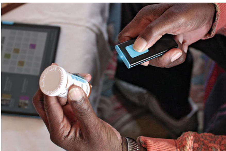
Fig. 10.3 Project HealthDesign is a program sponsored by the Robert Wood Johnson Foundation’s Pioneer Portfolio and intended to foster development of personal health records. Here is a barcode scanner that recognizes medication labels. Designed by researchers at the University of
