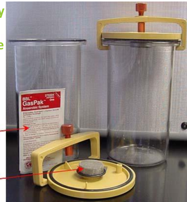
Wire mesh containing palladium catalyst
