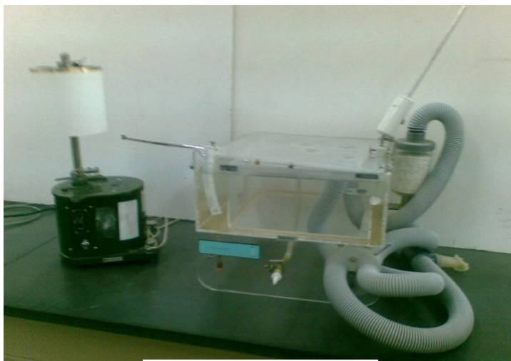
Simple (volumetric) spirometer.
