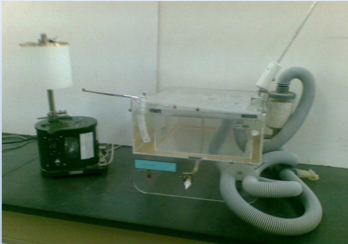
Simple (volumetric) spirometer.
