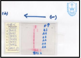
NAME THIS TEST? GEL ELECTROPHORESIS TEST
