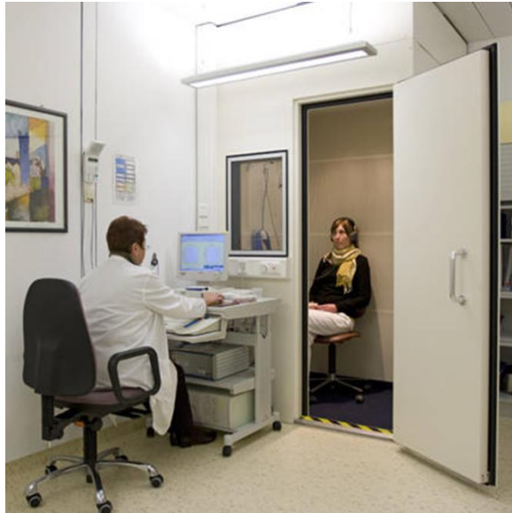
Figure 13. Hearing assessment using and audiometer with the study subject sitting in a sound proof room.
