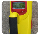
Ionization chamber in the machine to check if there is any leakage of radiation in the room which shielded with lead
