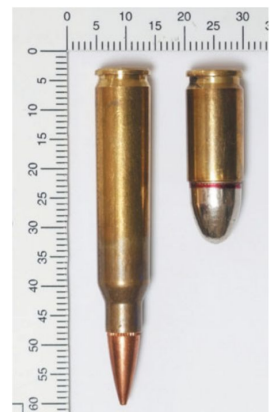
Figure 23.19 A 9 × 19 mm Luger semi-automatic pistol cartridge (top), and a NATO 5.56 × 45 mm automatic rifle cartridge (bottom).
