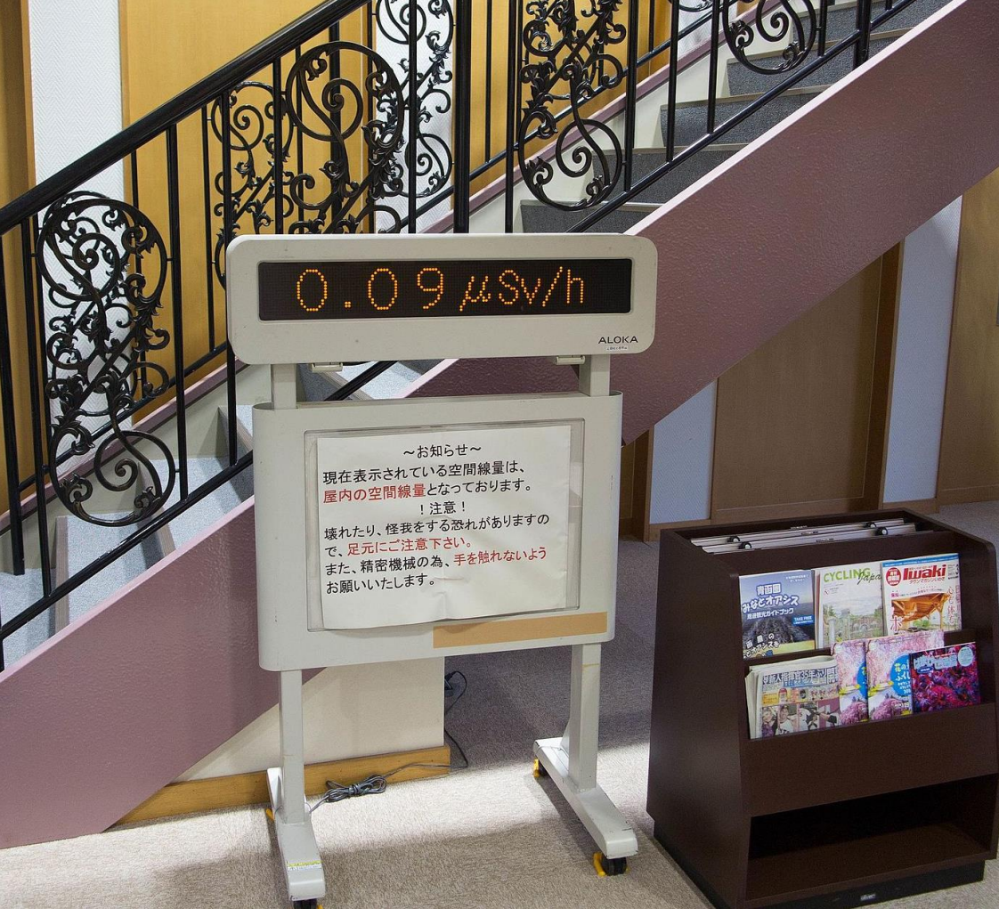
Display of background radiation in a hotel at Naraha, Japan, showing dose rate in microsieverts per hour, five years after the Fukushima disaster.
