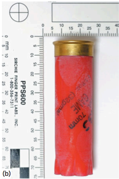
Figure 23.13 A fired shotgun cartridge: (a) untreated, and (b) treated with cyanoacrylate (superglue) fumes, revealing finger marks.
