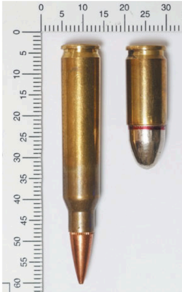
Figure 23.19 A 9 × 19 mm Luger semi-automatic pistol cartridge (top), and a NATO 5.56 × 45 mm automatic rifle cartridge (bottom).
