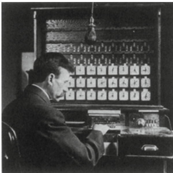
Fig. 1.12 Tabulating machines. The Hollerith Tabulating Machine was an early data-processing system that performed automatic computation using punched cards (Photograph courtesy of the Library of Congress.)
