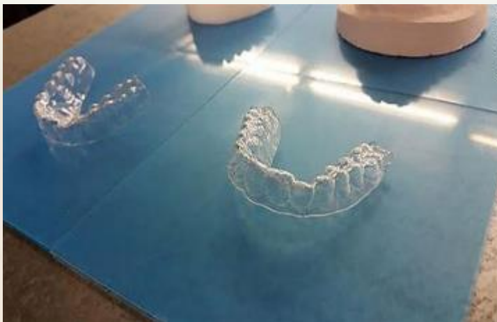
3D Printed In-house orthodontic aligners
