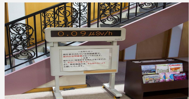
Display of background radiation in a hotel at Naraha, Japan, showing dose rate in microsieverts per hour, five years after the Fukushima disaster.
