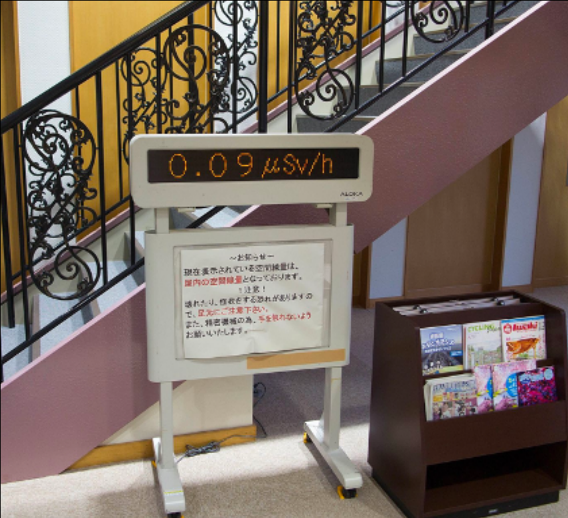
Display of background radiation in a hotel at Naraha, Japan, showing dose rate in microsieverts per hour, five years after the Fukushima disaster.
