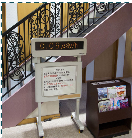
Display of background radiation in a hotel at Naraha, Japan, showing dose rate in microsieverts per hour, five years after the Fukushima disaster.
