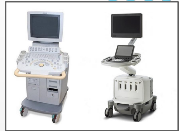
US Scanner mean frequency of 10 to 14mhz Transducer : linear
