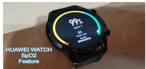
Smart watch with the ability to detect oxygen saturation
