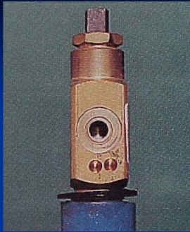
Nitrous cylinder valve and pin index
