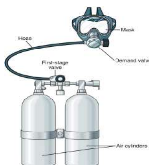
Figure 45-4. Open-circuit demand type of SCUBA.
